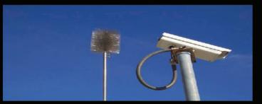
Each **Passive-Point Discharge element** contains up to 12,000 stainless steel points, which are arranged in such a manner to produce maximum ionization. The central twisted core of the unit is also made of stainless steel. The mounting bracket is fabricated and galvanized and each unit is hand-finished and inspected. A special lacquering process is employed which is unique to these units. This process assists in further protecting the unit from effects of the environment.
