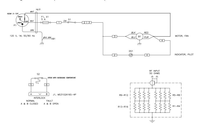
Figure 1. Power Circuit Schematic
