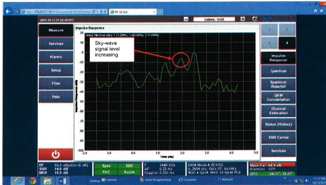
Figure 8: KinStar Antenna. Impulse response indicating increase in sky-wave level.
