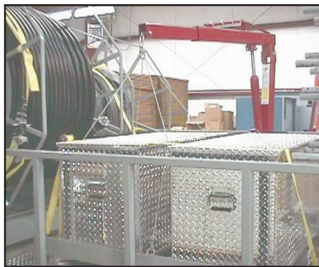
Photo 3: Hand crane lifting custom aluminum cargo boxes
