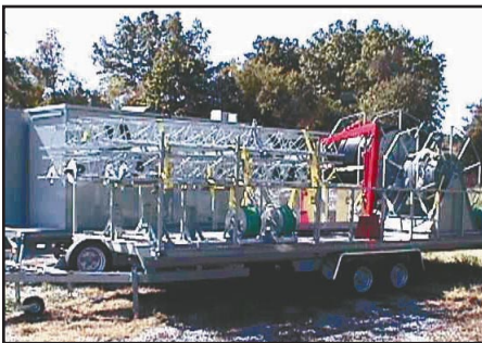
Photo 1: Antenna trailer loaded for travel
