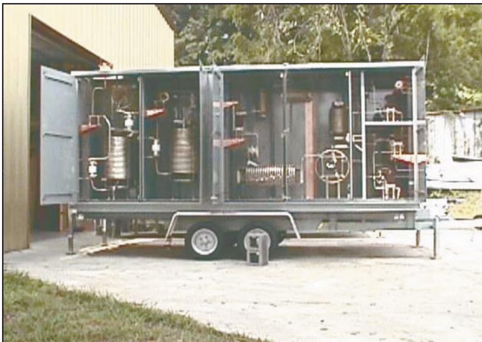
Photo 4: Interior of one triplexer unit
