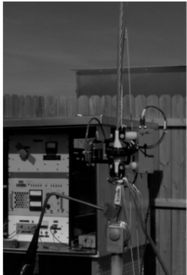
Figure 2. Measurement unit for taking current data on vertical wire. This unit is battery powered and consists of a sensing coil, measuring circuit, and digital storage unit. Transmitter visible in cabinet to rear.
