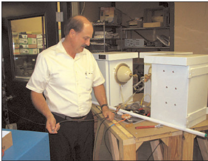
VSU-1 Voltage Sampling Units Under Test
