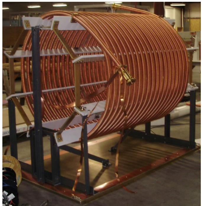
Fig 8 Isolation Coil for MediaFLO TV Facility at WJR
